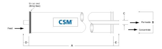
Each membrane element supplied with one brine seal, one interconnector (coupler) and four o-rings.
